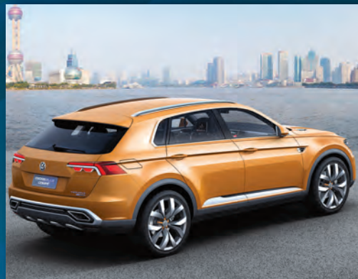
VW Crossblue Coupe: More crossover than coupe, this enviro-friendly VW can scoot from 0 to 60 mph in less than six seconds and has a 570-mile range—thanks to a robust V6 turbo and two electric motors.
