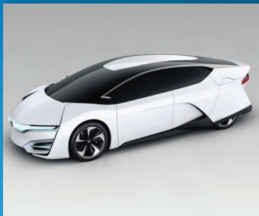
Honda FCEV: This five-seat fuel-cell electric vehicle—the successor to the FCX Clarity—has a coupe-like profile and range of 300 miles on a single fill-up of hydrogen.
